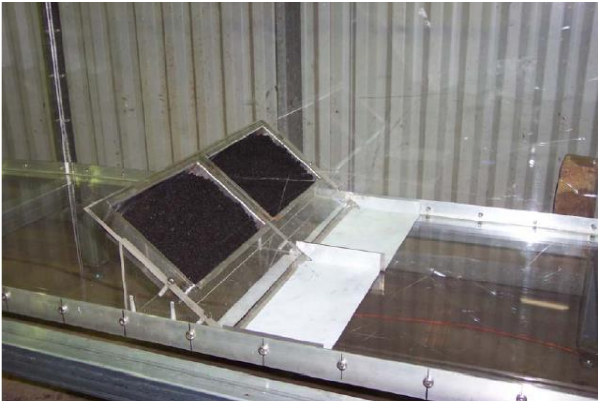
Figure 1: Wind tunnel with two sample trays
