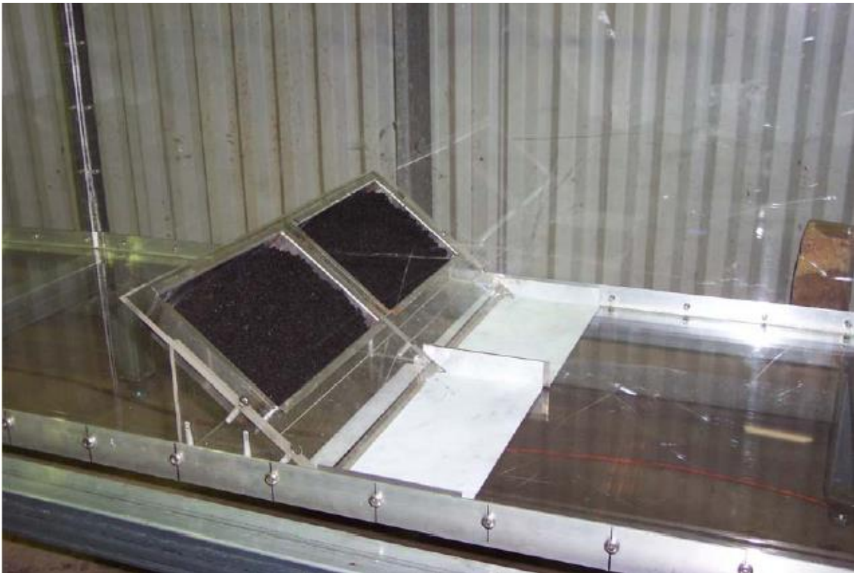
Figure 1: Wind tunnel with two sample trays containing typical coal type
